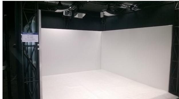
Fig. 1. Four-wall CAVE system with optical tracking cameras.
