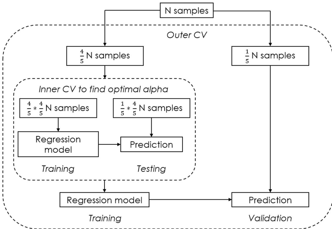
**Figure 2: Schematic overview of the developed prediction framework for feature (sub-)set validation.** The shown wrapper function consisting of an inner cross-validation, used to tune the hyperparameter alpha of the ridge regression algorithm, and an outer cross-validation to predict cognitive scores of the subjects and test the generalizability of the model. The process is repeated five times, so every subject has been part of the validation group exactly once.
